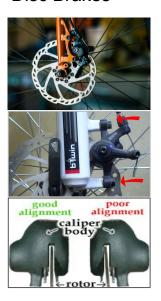
**To loosen:** Find both of the hex bolts that hold the brake caliper to the frame. Insert an Allen wrench of the corresponding size and twist it a half turn or more counterclockwise.
