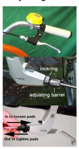
Regardless of the type of brake used, the brake pads should not drag against the rim and squeezing the lever should activate the brakes quickly.
