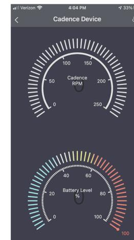
5. After the sensor is connected, you can use the App to check the battery level and RPM directly from the sensor. (Turn the crank to see the Cadence RPM change)
