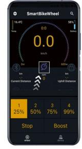
The highlighted crank icon indicates the cadence sensor is connected
